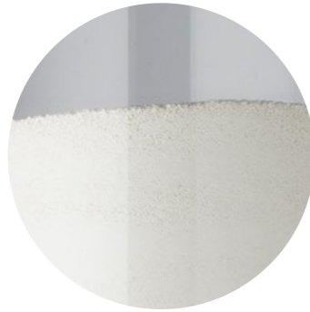
pressing granules the hollow granules are being used for the production of the plates
